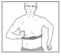
tor should be under your clothing, tight against your skin, and as high under the pectoral muscles or breasts as is comfortable. Make sure that the logo on the sensor unit is facing forward and is right-side-up.
